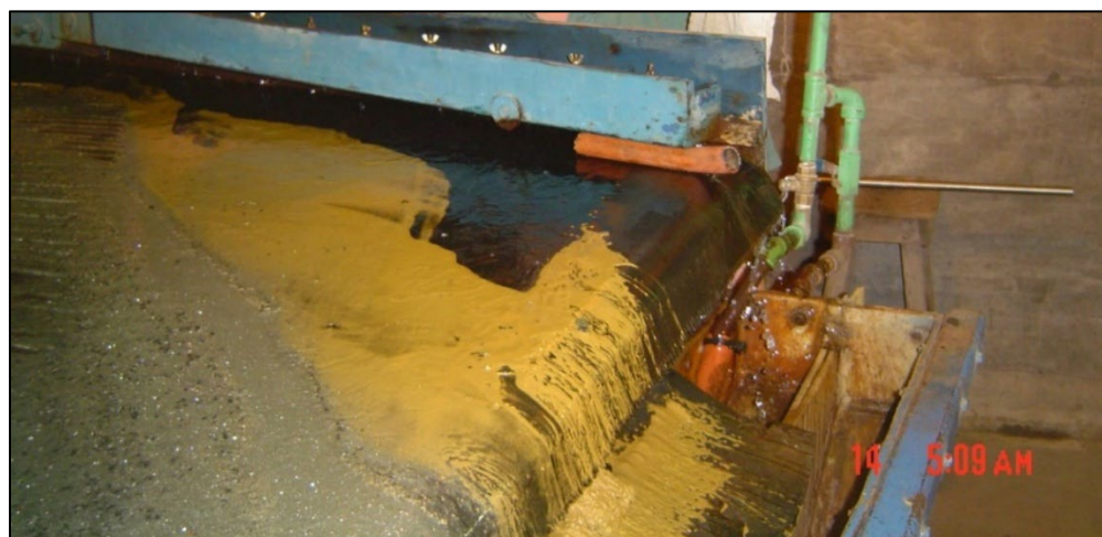
FIGURE 13.2 GOLD CONCENTRATION ON SHAKING TABLE
