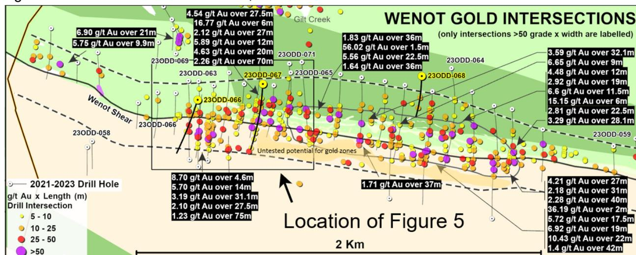
Further downhole in 23ODD-066, a 75-m wide sediment-hosted shear includes 5.89 g/t Au over 8.7m, 0.9 g/t over 13.0m, 0.40 g/t over 14.6m, 0.45 g/t over 7.9m. Approximately 50m above hole -066, an older drill hole intersected the same zone, returning 1.23 g/t Au over 75.0m. Previous shallow drill holes show continuity of this zone to surface. Further to the west, there is limited drilling and focused on the central contact shear and the volcanic sequence to the north.
